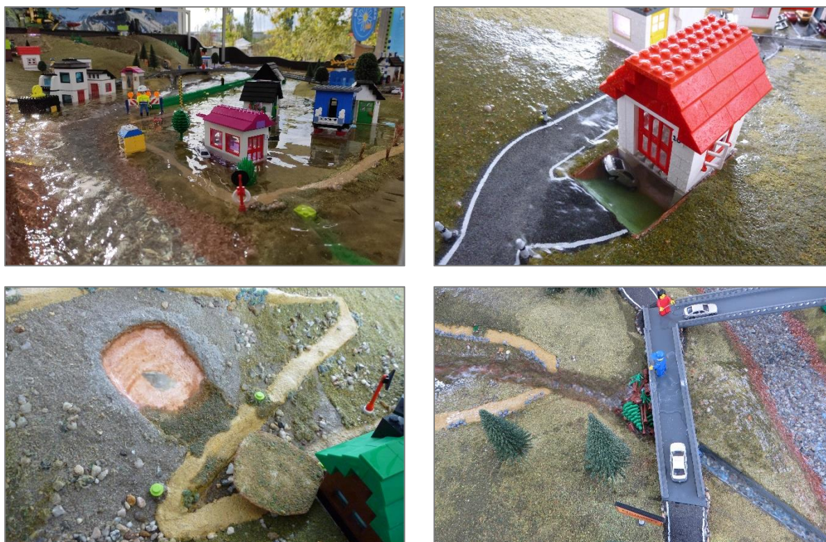
Figure 11: Model landscape of the natural hazard model: simulation of floods along the river course with a water pump, simulation of heavy rain and surface discharge with water nozzles, activation of a slide with a water hose and a loose plate, and release of a torrent with a water hose causing a debris jam © Bavarian Environment Agency
