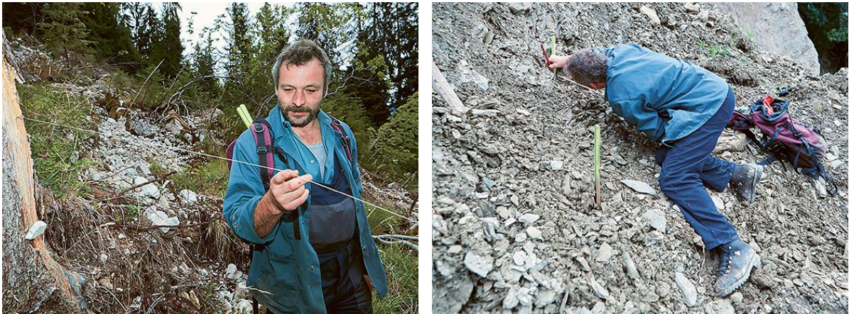
Figure 8: With the help of fixed points, the natural hazard advisor can recognise changes in the terrain at risk of slipping. Among other things, he places flags and wooden slats in the terrain as reference points. © Ephraim Bieri/BAFU
